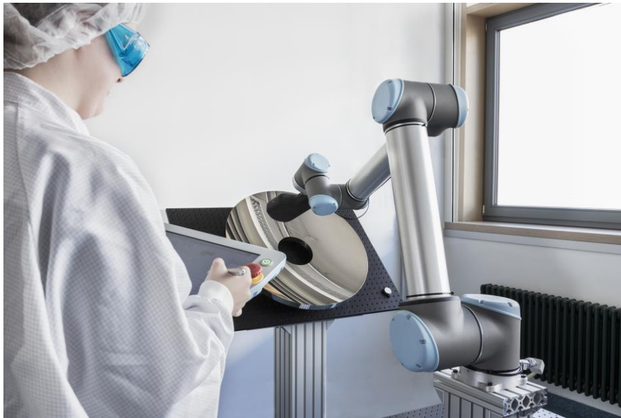
Image 2) Robot-supported scattered light measurement. (©Fraunhofer IOF)
