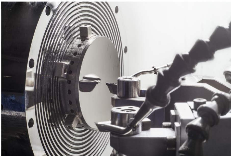
Image 3) UP-machining of an additive manufactured light weight mirror. (©Fraunhofer IOF)
